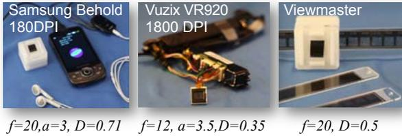
**Figure 8:** Three of our prototypes: (left) cell phone, (center) high-resolution display, (right) View-Master.
